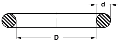
O-Ring NBR 90 Sh A – FPM 90 Sh A
